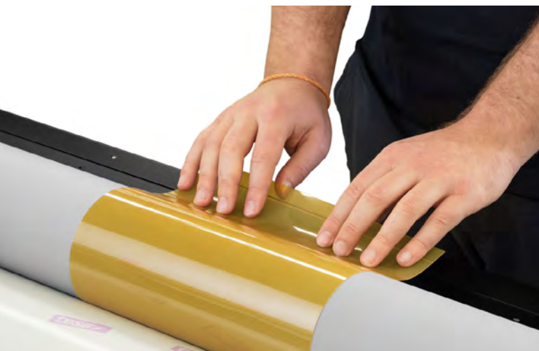
Pressure roller that creates friction without damaging the plate
