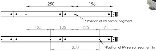
Position of HV sensor, segment in reverse position
