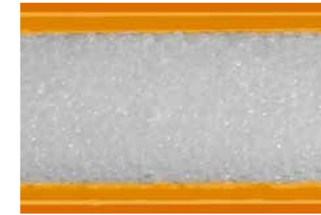
Cross-section 3-layer sheet with a foamed middle layer
