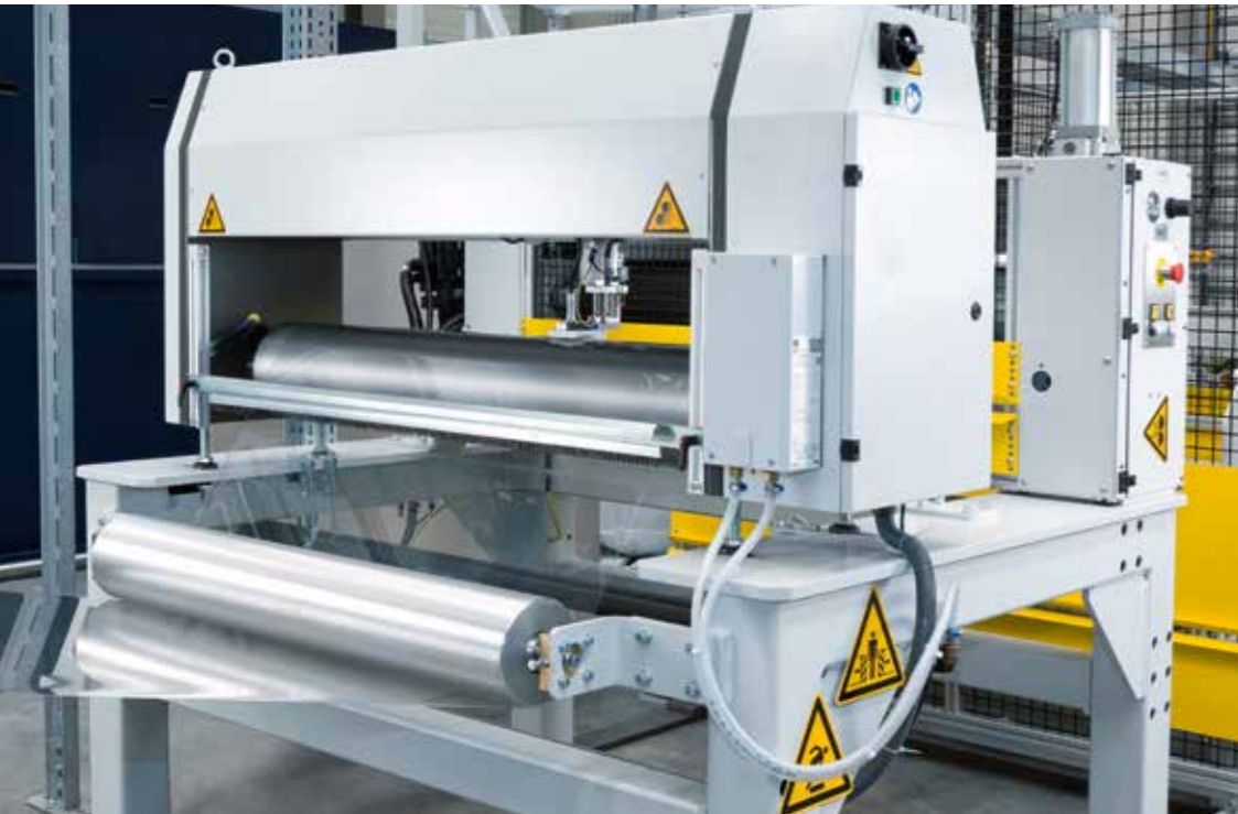
Inline thickness-measuring unit with an inductive / capacitive sensor
