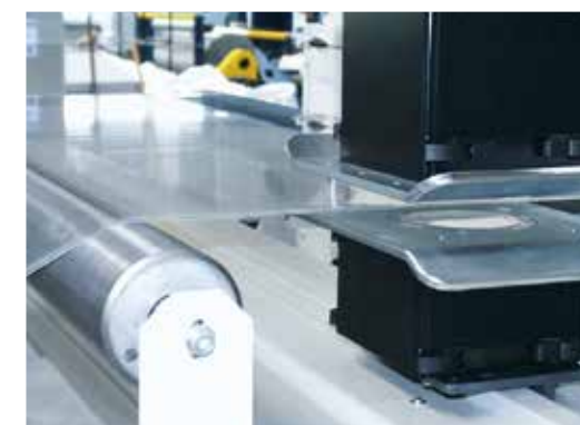
inline thickness measuring unit with Beta-ray sensor
