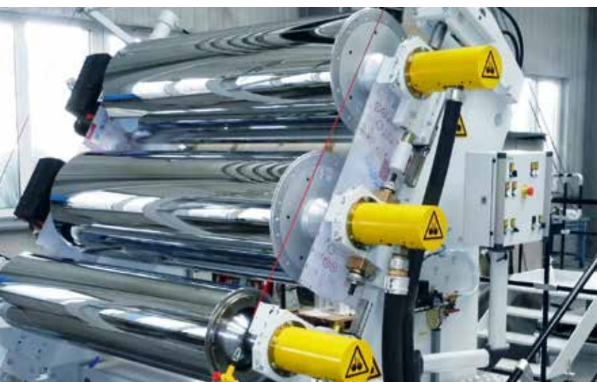
inclined roll stack
