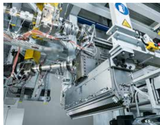
tool unit with melt pump, static mixer, feedblock and flat die
