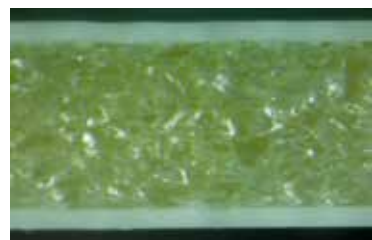
Cross section 3-layer sheet with foamed middle layer
