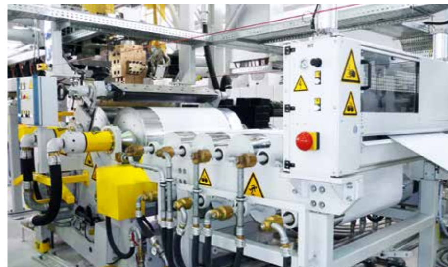
horizontal roll stack with additional cooling rolls
