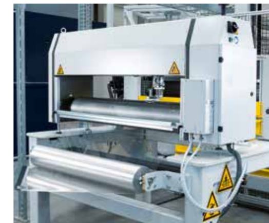
inline thickness measuring unit with inductive/capative sensor
