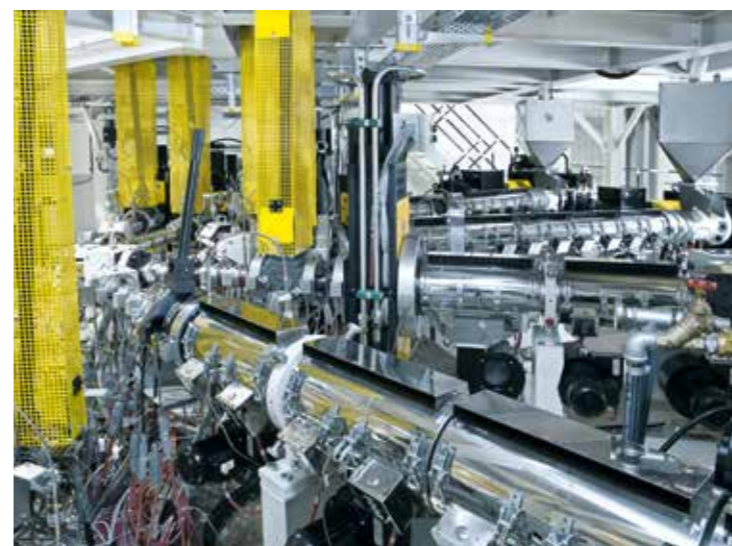
extruder arrangement of a barrier sheet line
