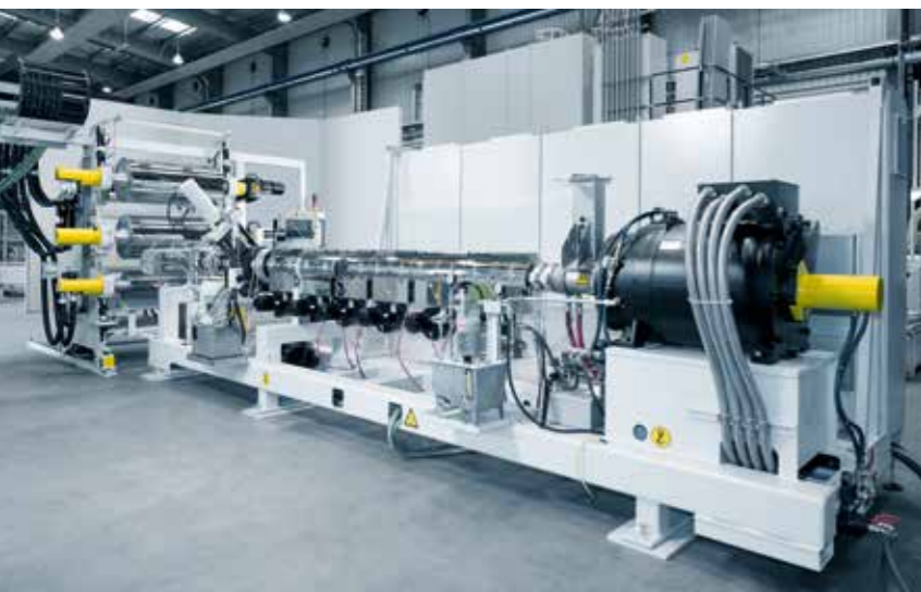
I-TF3 inline compact extrusion system with HSE90
